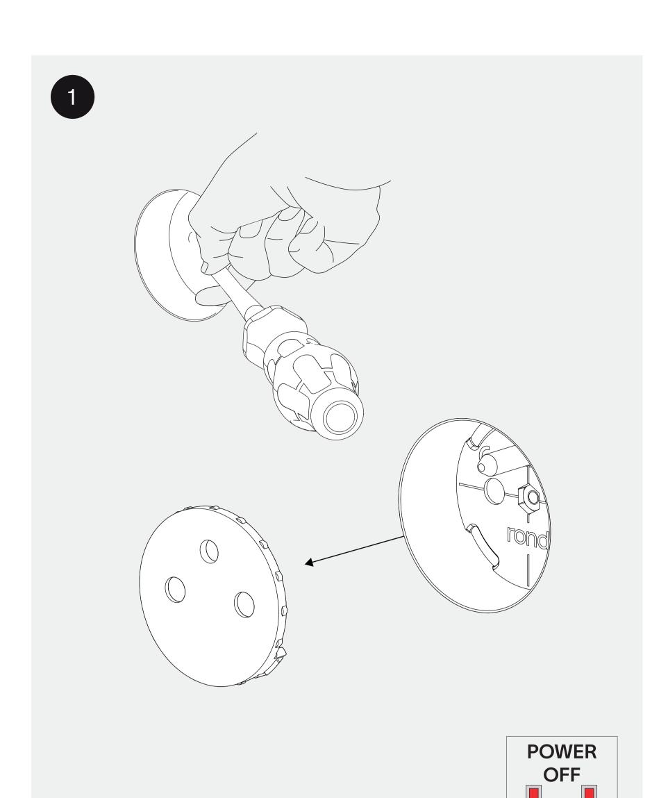
Gently remove the cover plate using a screwdriver. Place your finger between the screwdriver and the edge of the socket to prevent damaging the socket. Make sure the power is turned off before removal.
