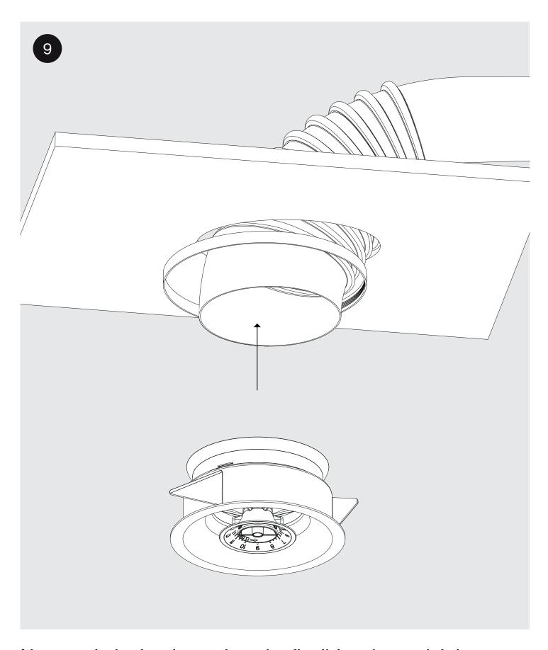
Now push the back part into the flexible tube and tighten the hose clamp.
