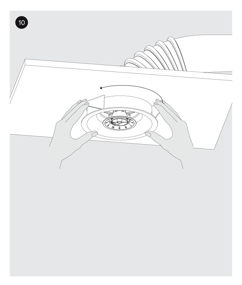
Push the valve into the ceiling opening while turning it.
