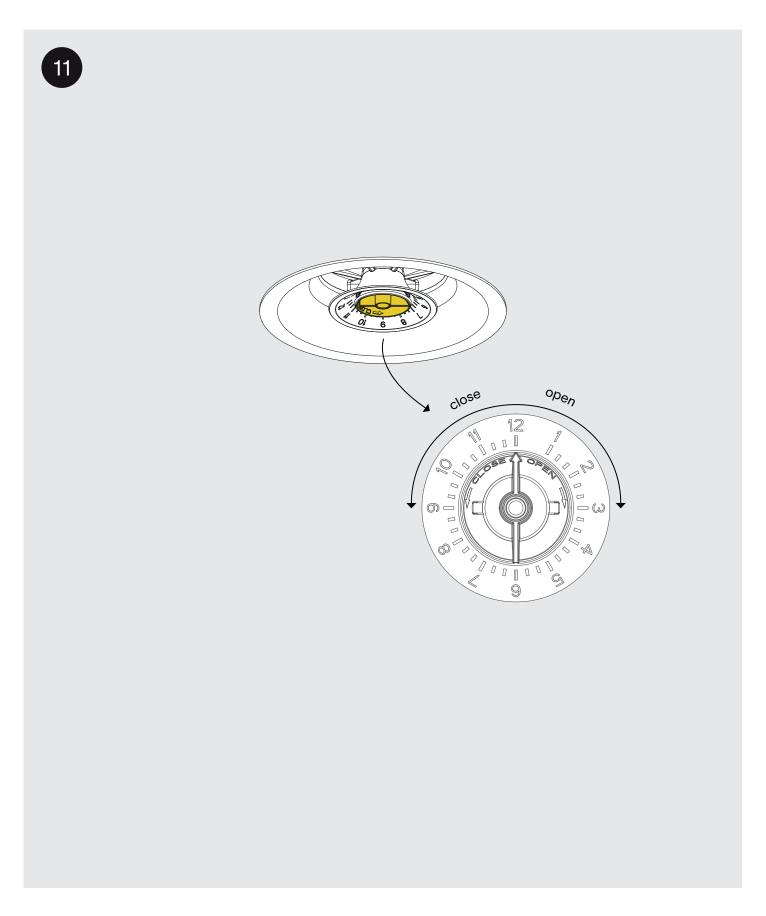
Twist the center of the valve to adjust the ventilation flow level.
