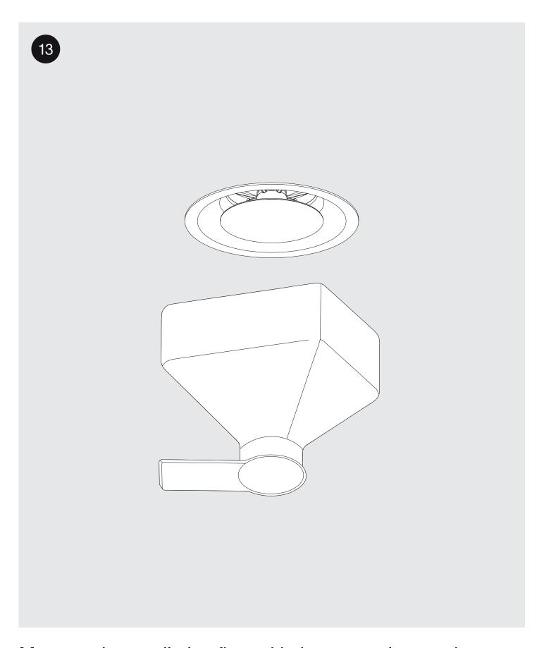
Measure the ventilation flow with the cover plate on the valve and repeat step 12 until the desired flow is reached.
