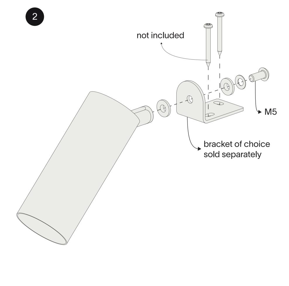
Install the fixture in the desired location.
