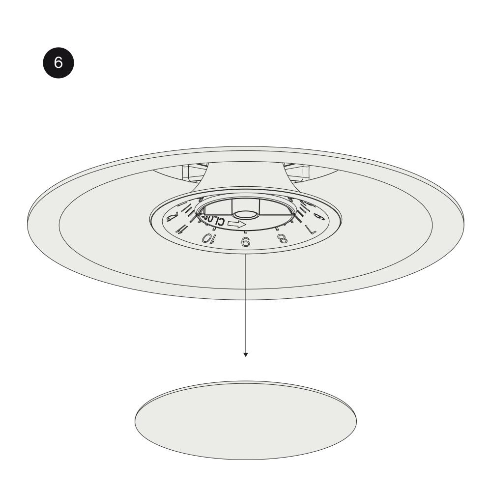
Remove the cover plate to adjust the ventilation flow.
