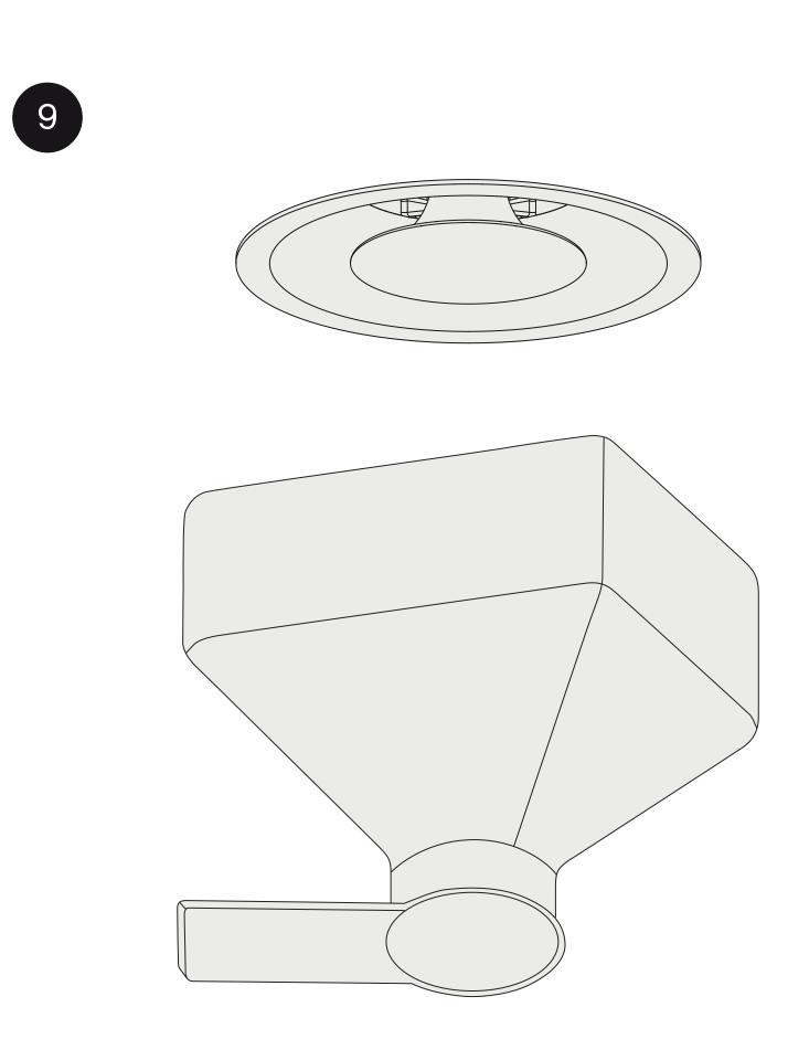
Measure the ventilation flow with the cover plate on the valve and repeat step 6 to 8 until the desired flow is reached.
