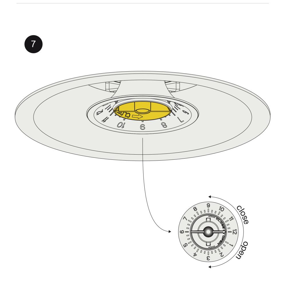
Twist the centre of the valve to adjust the ventilation flow level.
