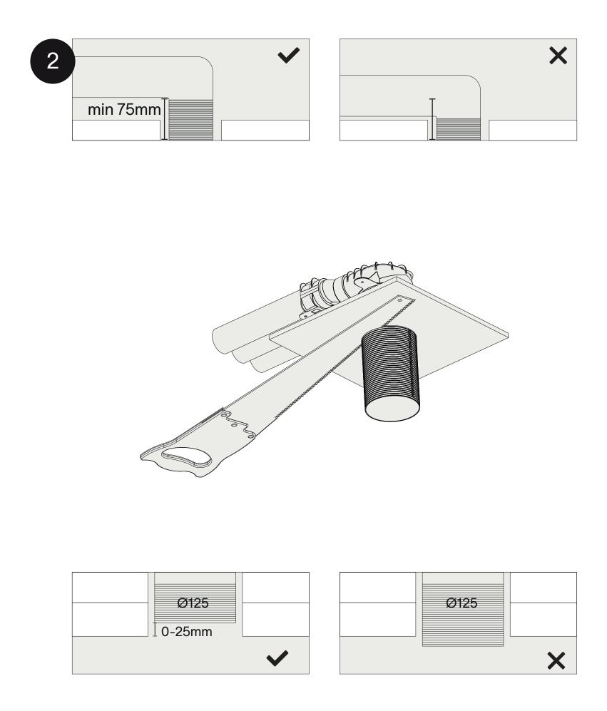
Cut off the excess length of the valve adapter. (between 0 and 25 mm above final ceiling level) The remaining vertical part of the adapter (before the start of the turn) must be at least 75 mm high for the ventilation valve. The valve is not compatible with a flexible ventilation duct.
