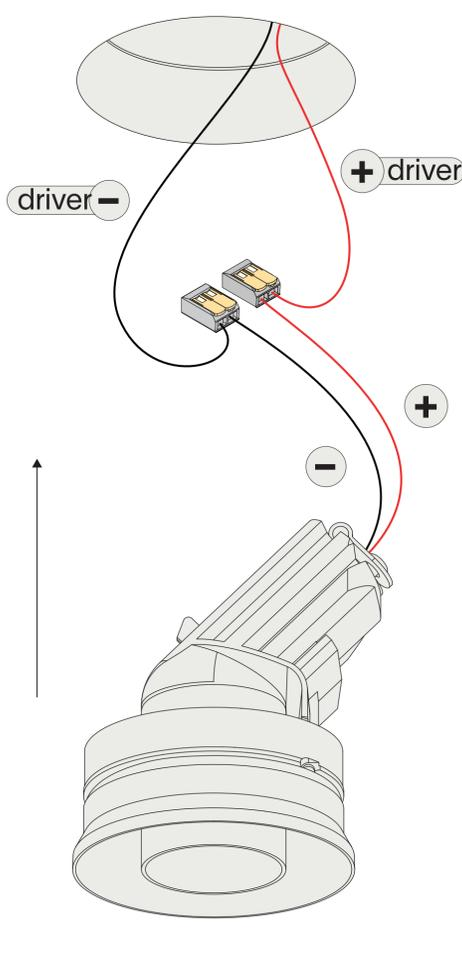
Connect the wires with the included connectors.
