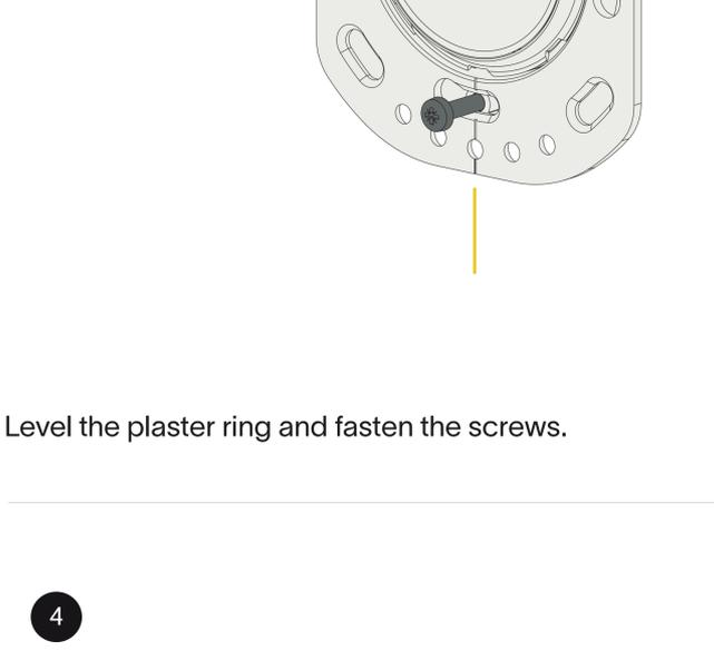
Level the plaster ring and fasten the screws.
