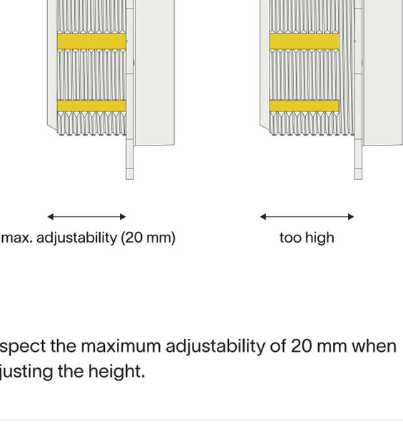
Respect the maximum adjustability of 20 mm when adjusting the height.
