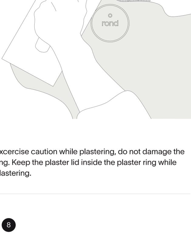
Exercise caution while plastering, do not damage the ring. Keep the plaster lid inside the plaster ring while plastering.
