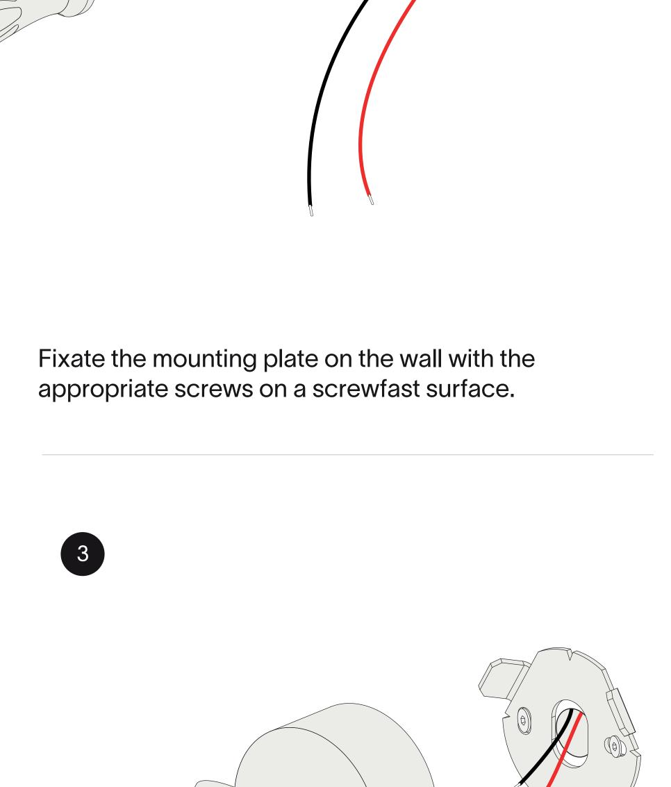
Connect the wires with waterproof connectors,
