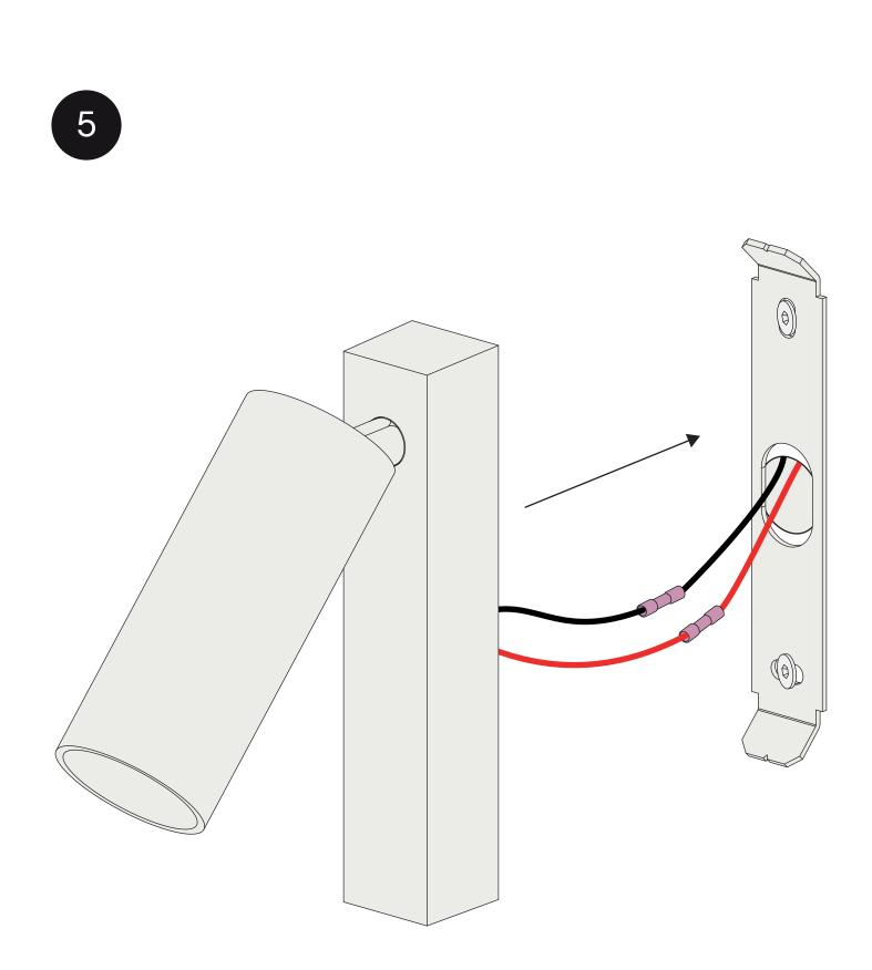
Click the fixture onto the mounting plate.
