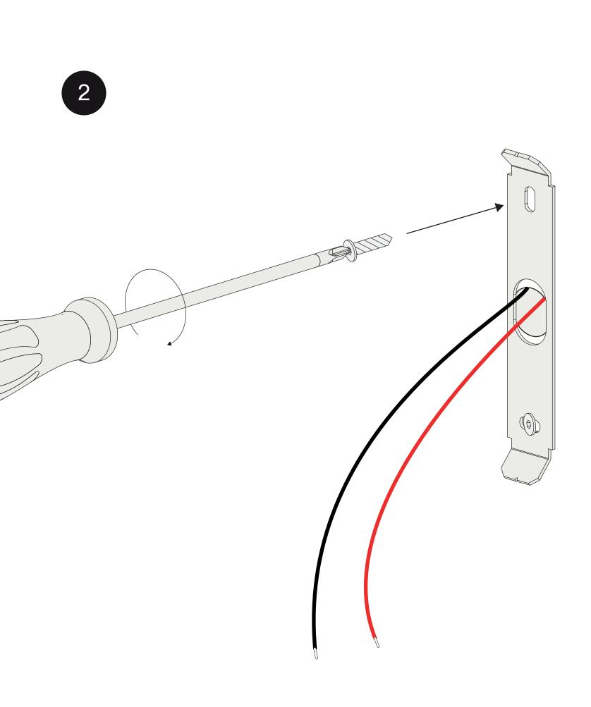
Fixate the mounting plate on the wall with the appropriate screws on a screwfast surface.
