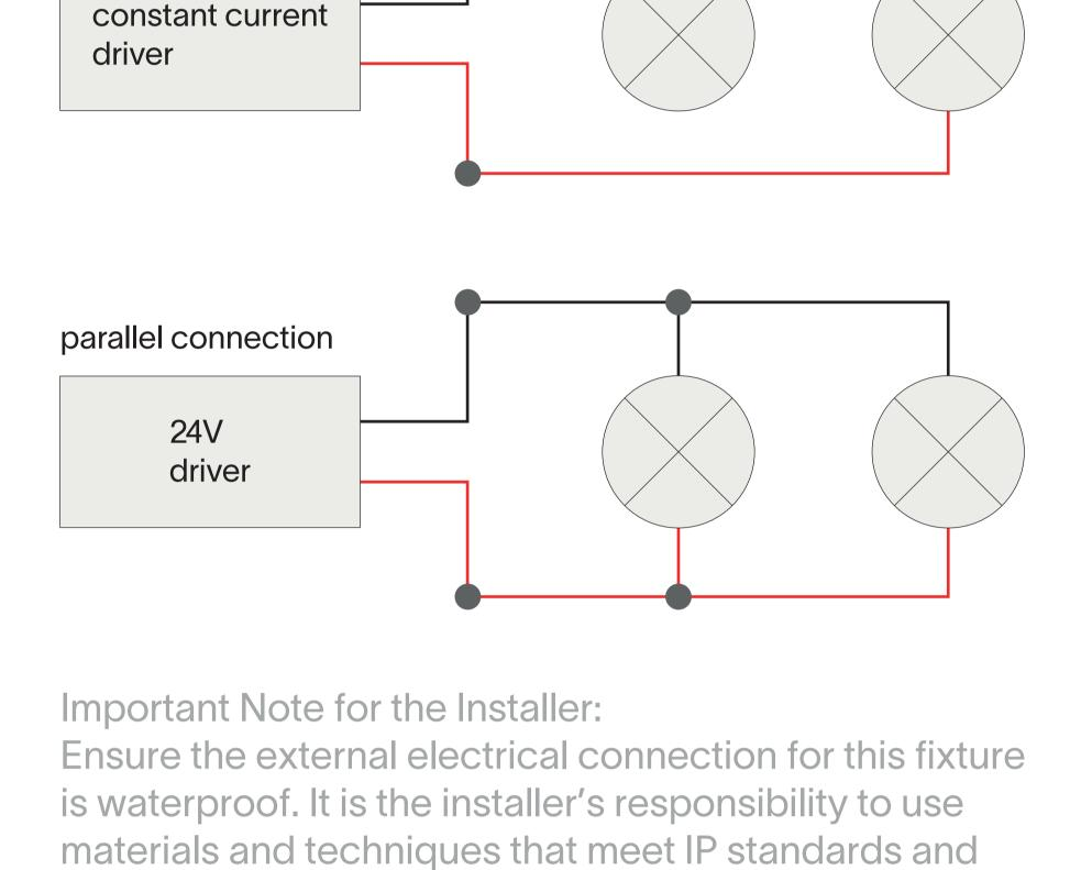
prevent water ingress. Failure to waterproof the
