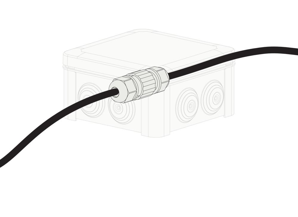
for 24V driver: parallel connection The installer is responsible for using the correct wire section and must consider the maximum cable length
