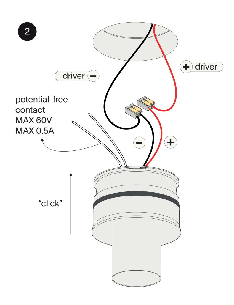
for parallel connection, respect polarity. Combine with a prado LED-driver. Gently click the luminaire into the plasterkit. The potential-free contact closes when the luminaire turns on.
