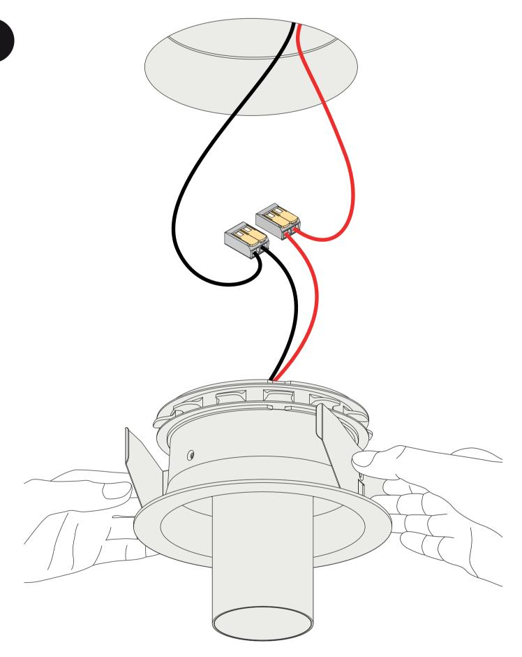
Bend over the springs and push the luminaire into the ceiling.
