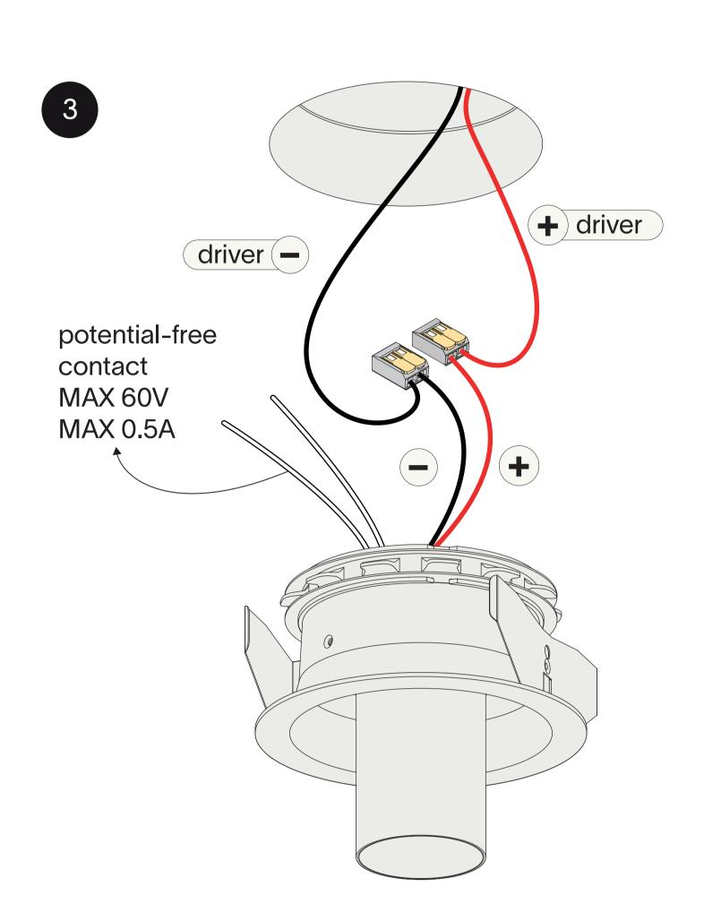
Connect the wires with wago connectors for parallel connection, respect polarity. Combine with a prado LED-driver. The potential-free contact closes when the luminaire turns on.
