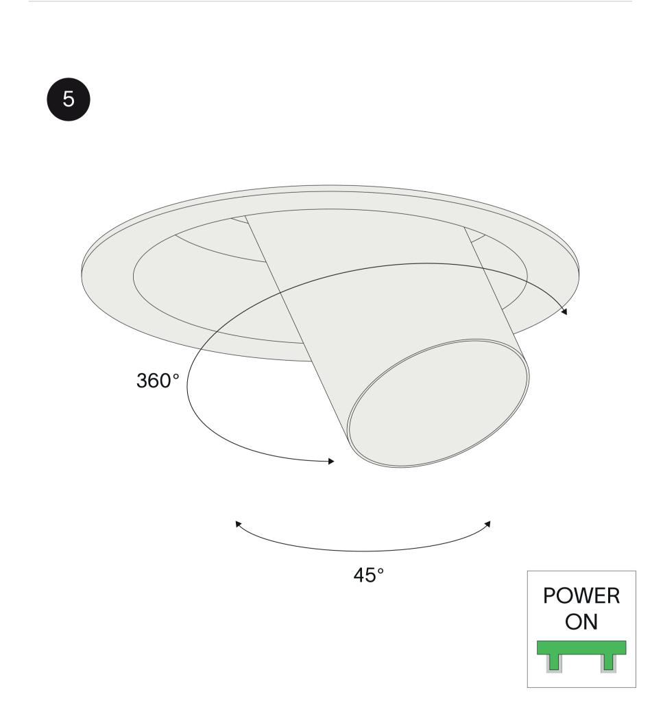
Turn the power back on. The luminaire will turn on when the ambient light is low enough and movement is detected. After the last detection of movement, the luminaire will stay on for 5 minutes. These are default settings and cannot be adjusted. Twist the luminaire as desired.
