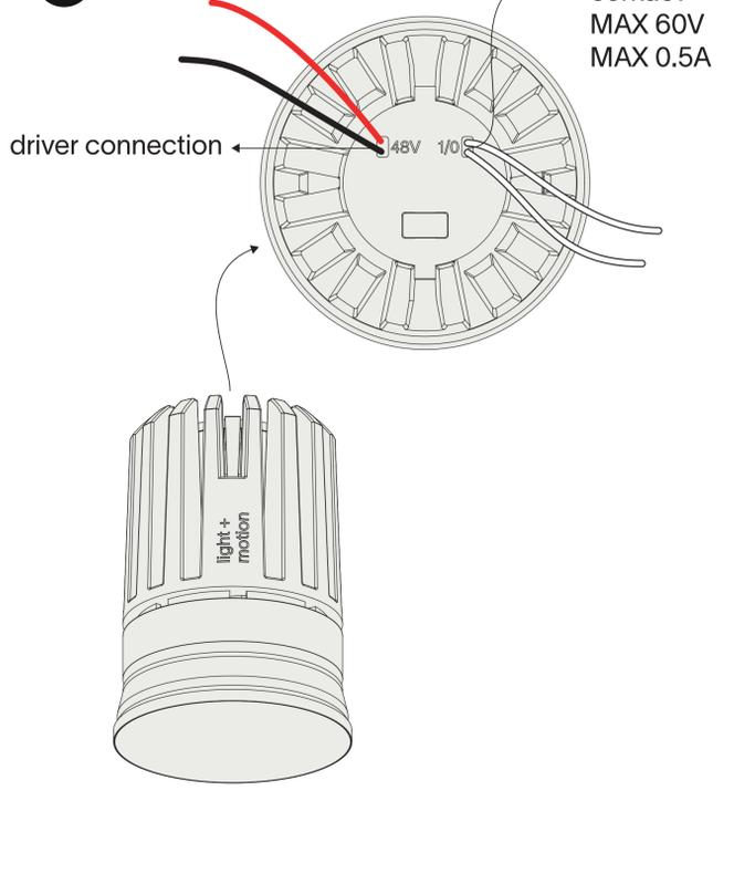
The potential-free contact closes when the luminaire turns on.
