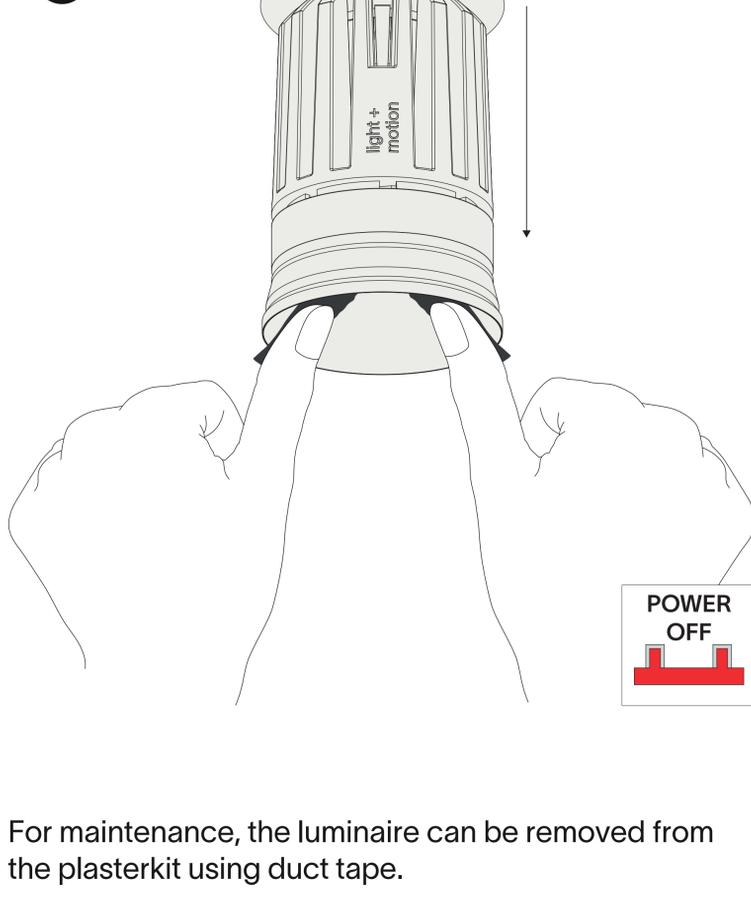
For maintenance, the luminaire can be removed from the plasterkit using duct tape.
