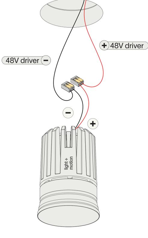
Connect the wires with wago connectors for parallel connection, respect polarity. Combine with a prado LED-driver.
