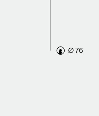
Cut a round hole (Ø 76). Consult the chosen luminaire tech specs for required height and free air dimensions.
