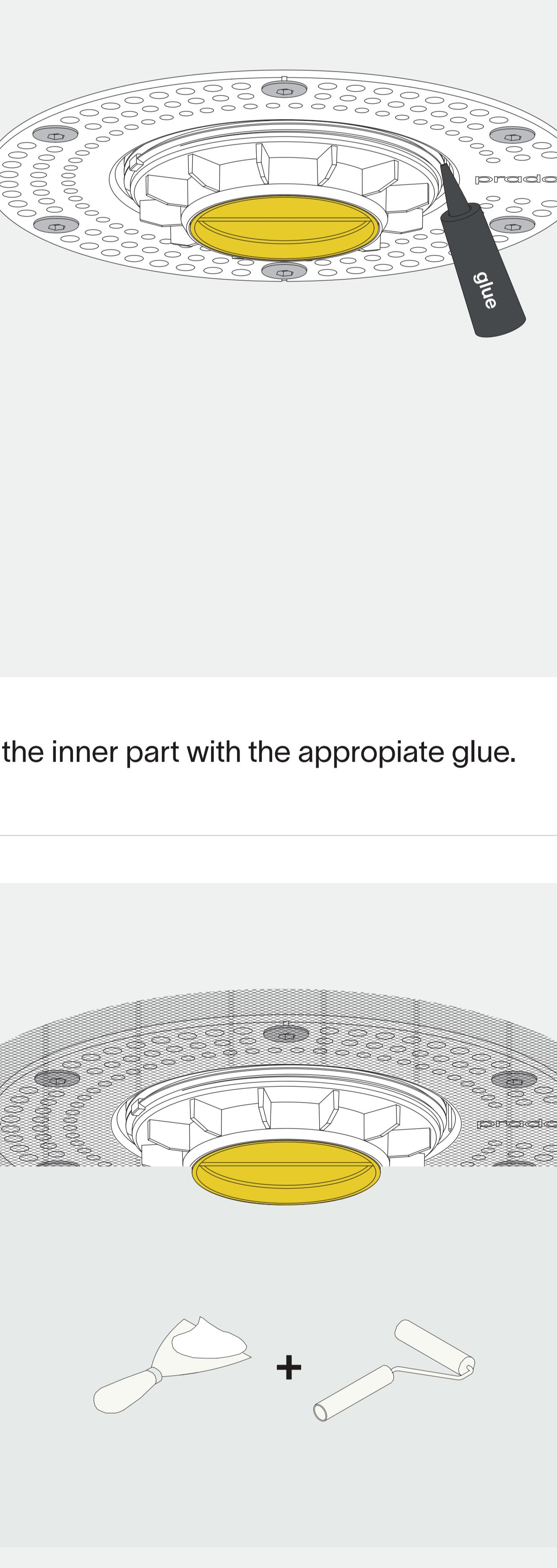
Insert the plaster ring and securely fasten it with glue or the appropriate screws on a screwfast surface. The attachment must be able to obtain a static load of 5 kg. It's the installers responsibility to ensure optimal attachment.
