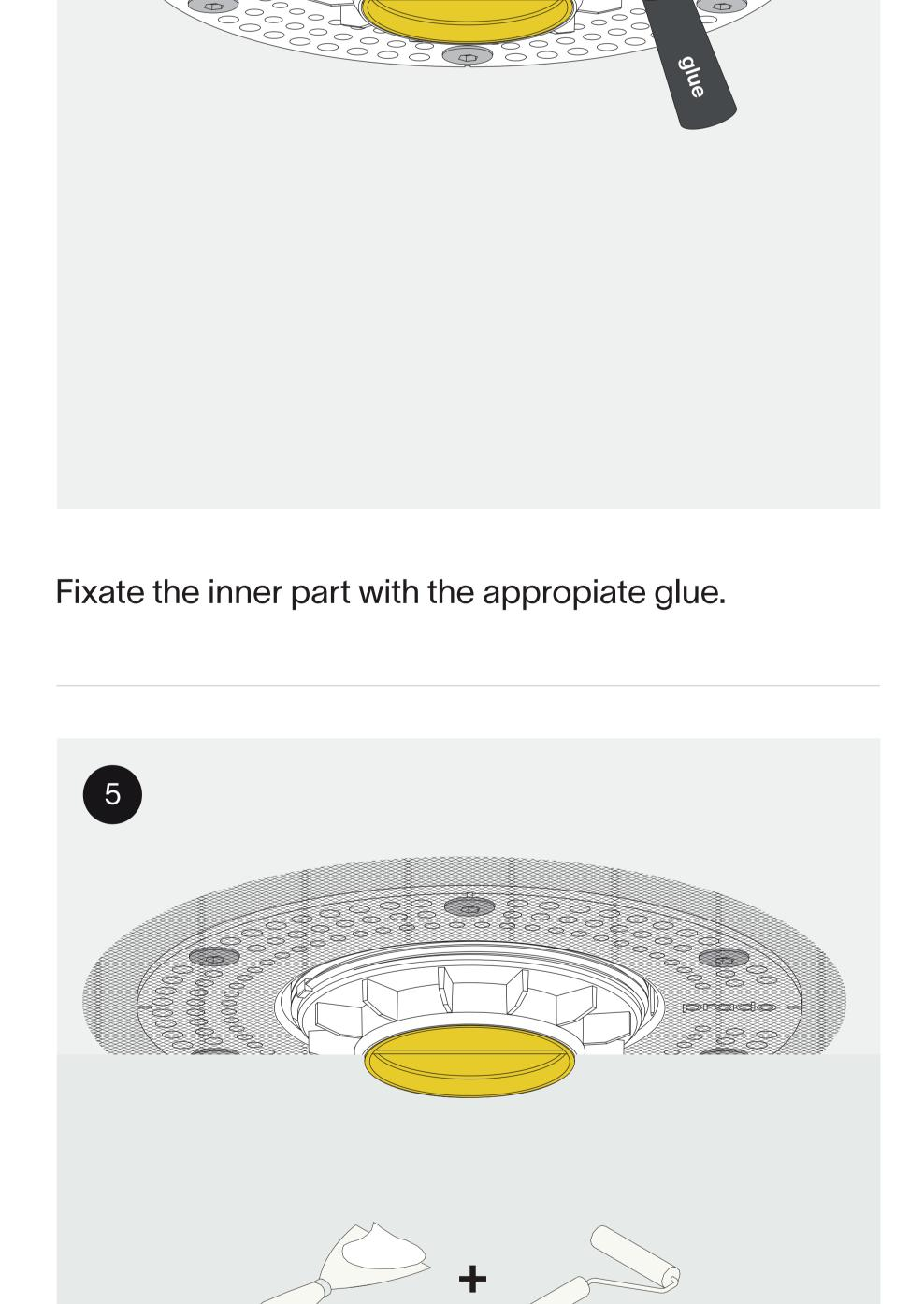
screwfast A surface plaster board perfect amount of plaster not enough plaster too much plaster Excercise caution while plasering, do not damage the ring. Keep the plaster lid inside the plaster ring while plastering. Use a fiberglass mesh tape for optimal plaster adhesion. Make sure not to touch the edge of the ring when sanding.
