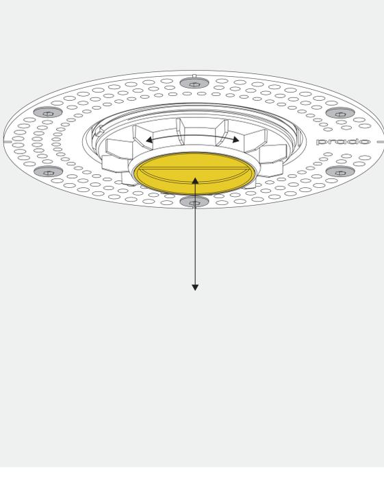
Adjust the height of the plaster ring by twisting the inner part of the kit (min. 3.6mm - max. 20mm).
