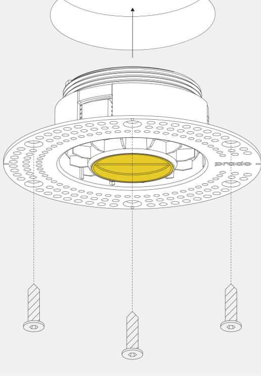
Insert the plaster ring and securely fasten it with glue or the appropriate screws on a screwfast surface. The attachment must be able to obtain a static load of 5 kg. It's the installers responsibility to ensure optimal attachment.
