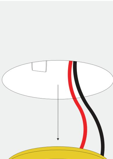
Remove the plaster lid before installing the fixture. Any residue needs to be removed without damaging the edges of the ring.
