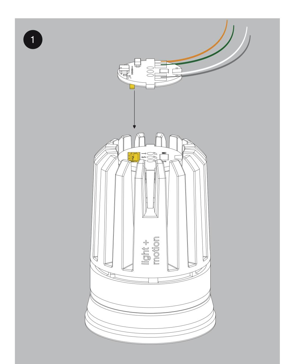
connect the relay accessory by connecting the male and the female side of the connector
