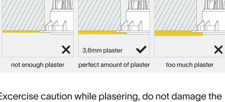
Excercise caution while plasing, do not damage the ring. Keep the plaster lid inside the plaster ring while plastering. Use a fiberglass mesh tape for optimal plaster adhesion. Make sure not to touch the edge of the ring when sanding.
