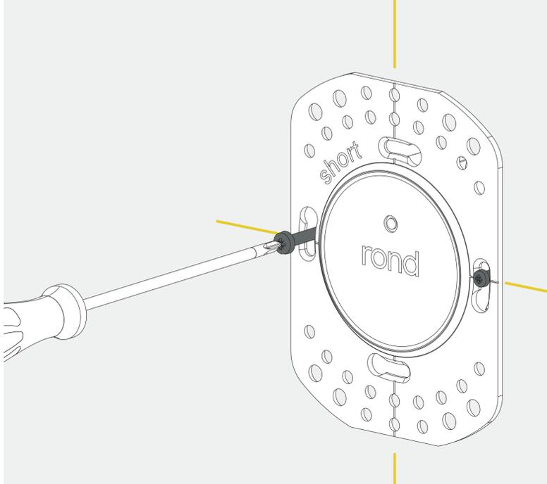
level kit, gently screw with appropriate stainless steel screws
