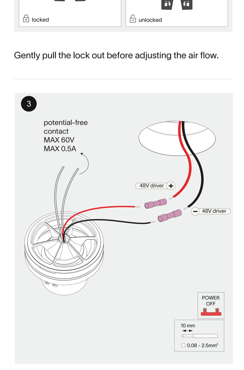
Connect the wires with waterproof connectors
