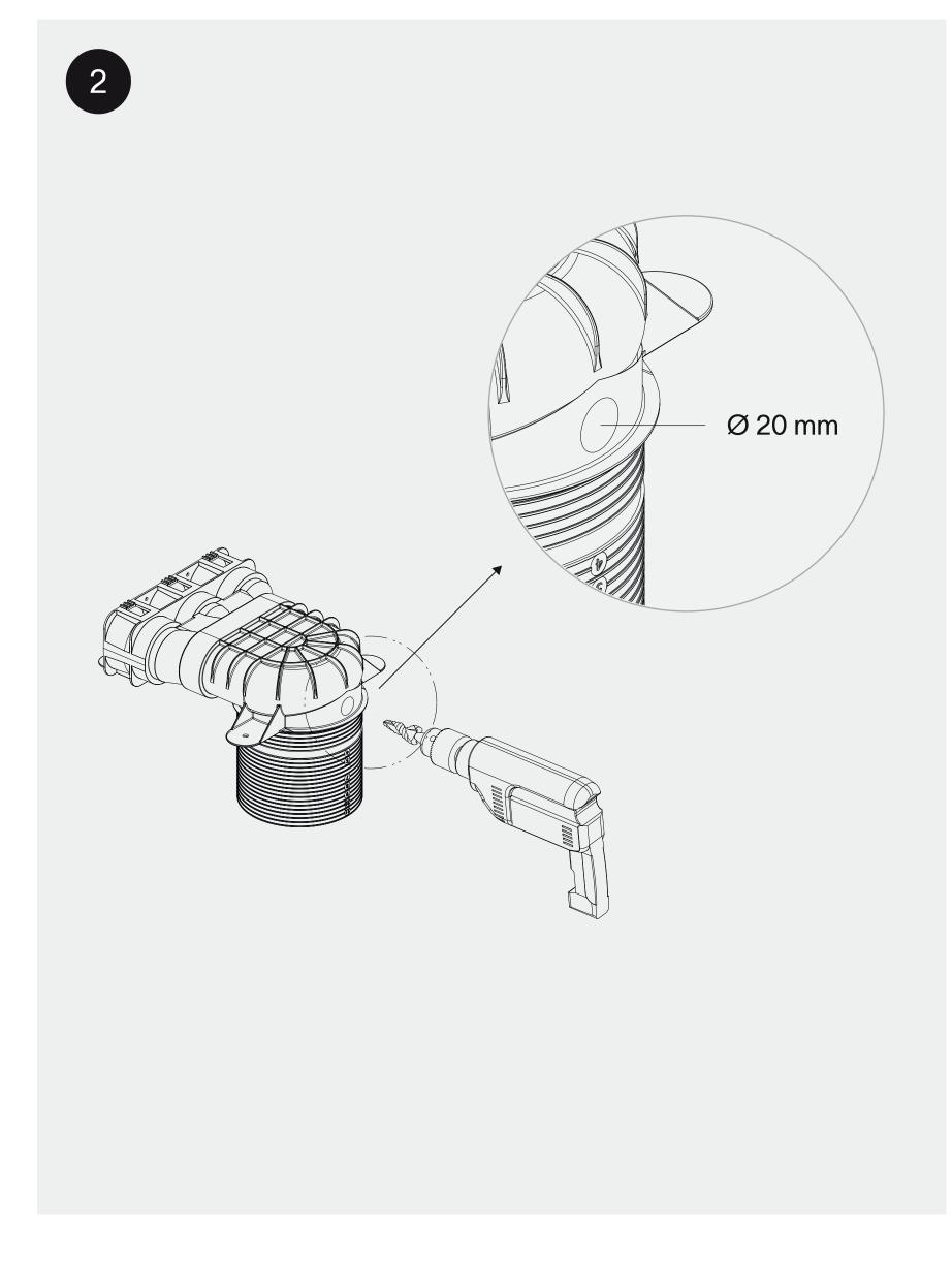
Use a step drill to cut a Ø20 hole into the Ø125 valve adapter of your choice. A hole can be drilled in any type or brand of Ø125 valve adapter.
