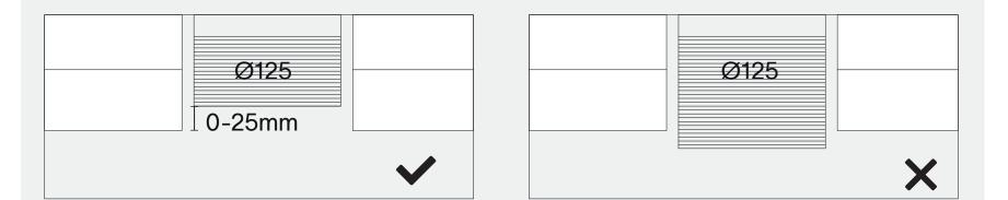
Cut off the excess length of the valve adapter. (between 0 and 25 mm above final ceiling level) The remaining vertical part of the adapter (before the start of the turn) must be at least 75 mm high for the plaster ring (connector can't be placed in this zone).
