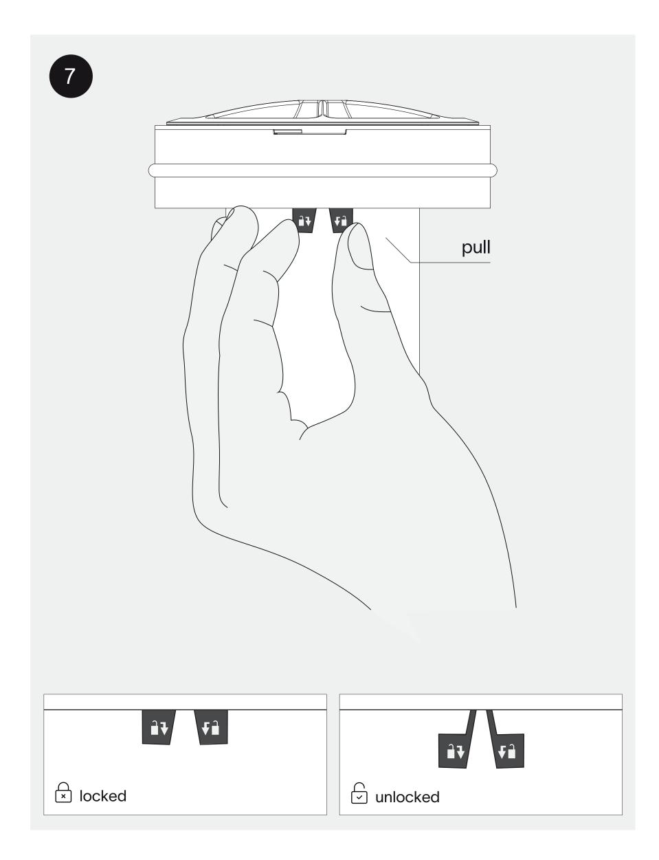
gently pull the lock out before adjusting the air flow
