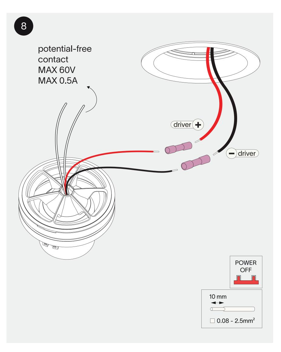
connect the wires with waterproof connectors for serial connection, respect polarity combine with prado LED-driver
