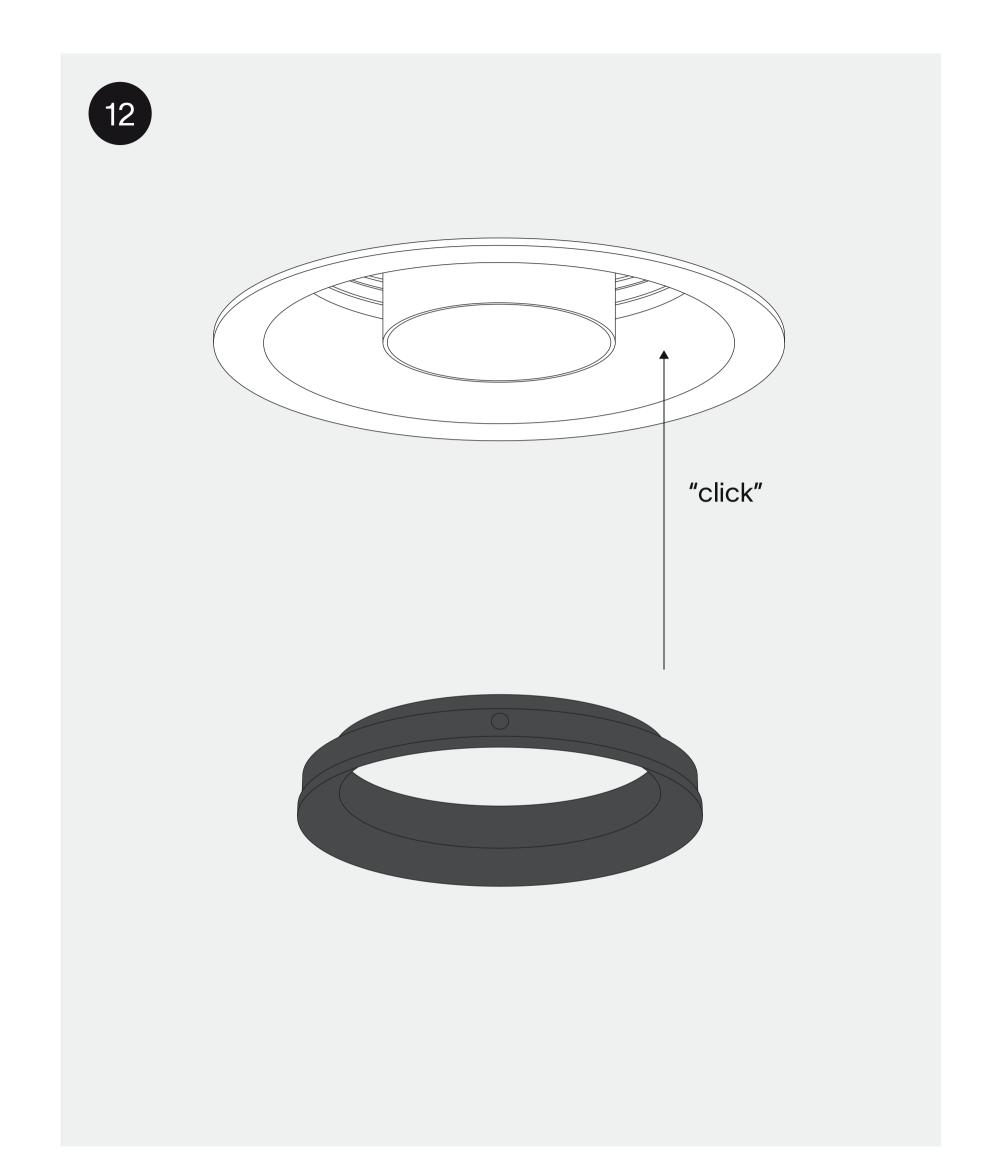
insert the design ring to lock the ventilation valve
