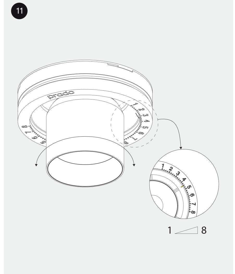
twist the luminaire to adjust the ventilation flow level
