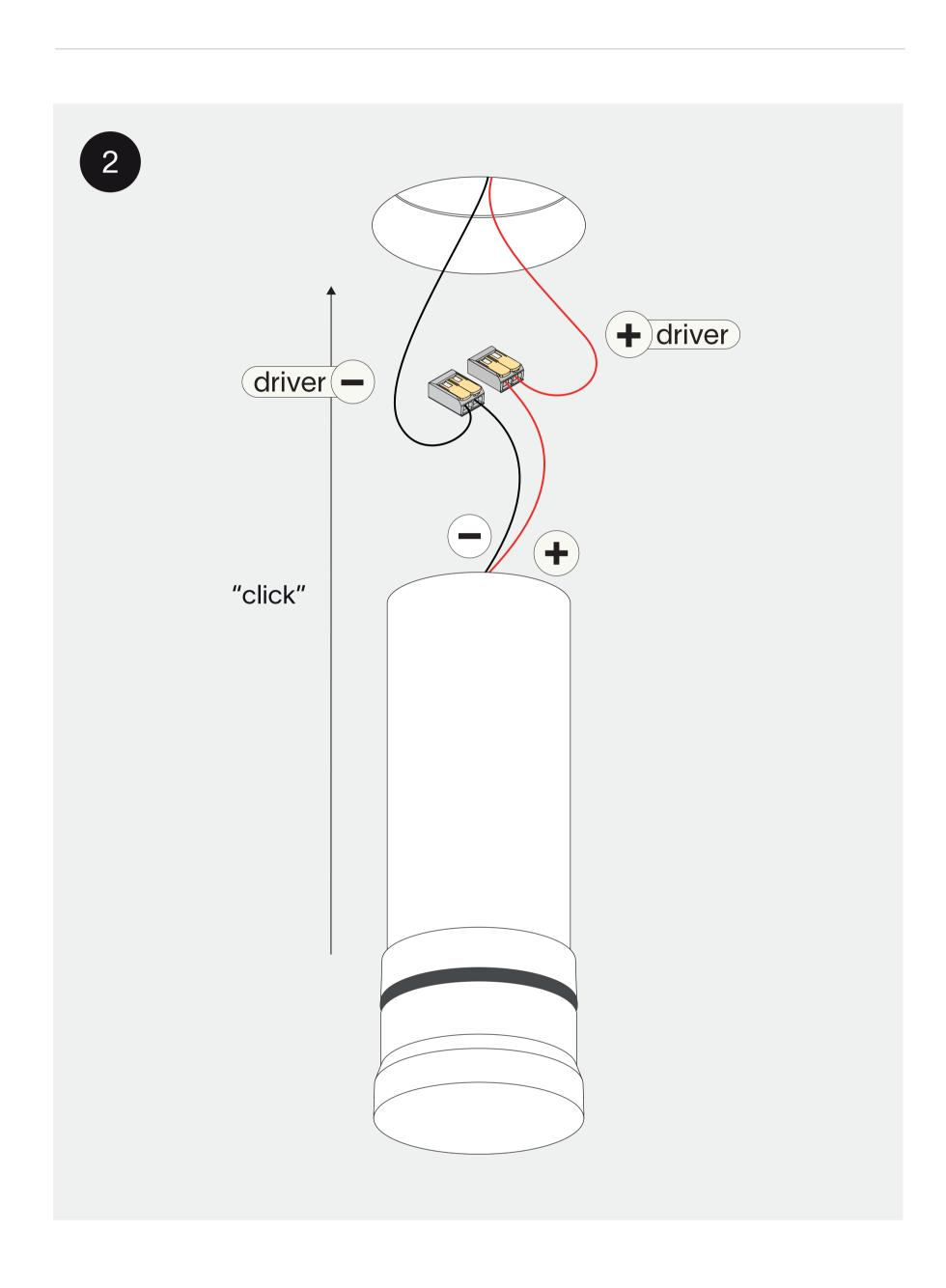
connect the wires with wago connectors
