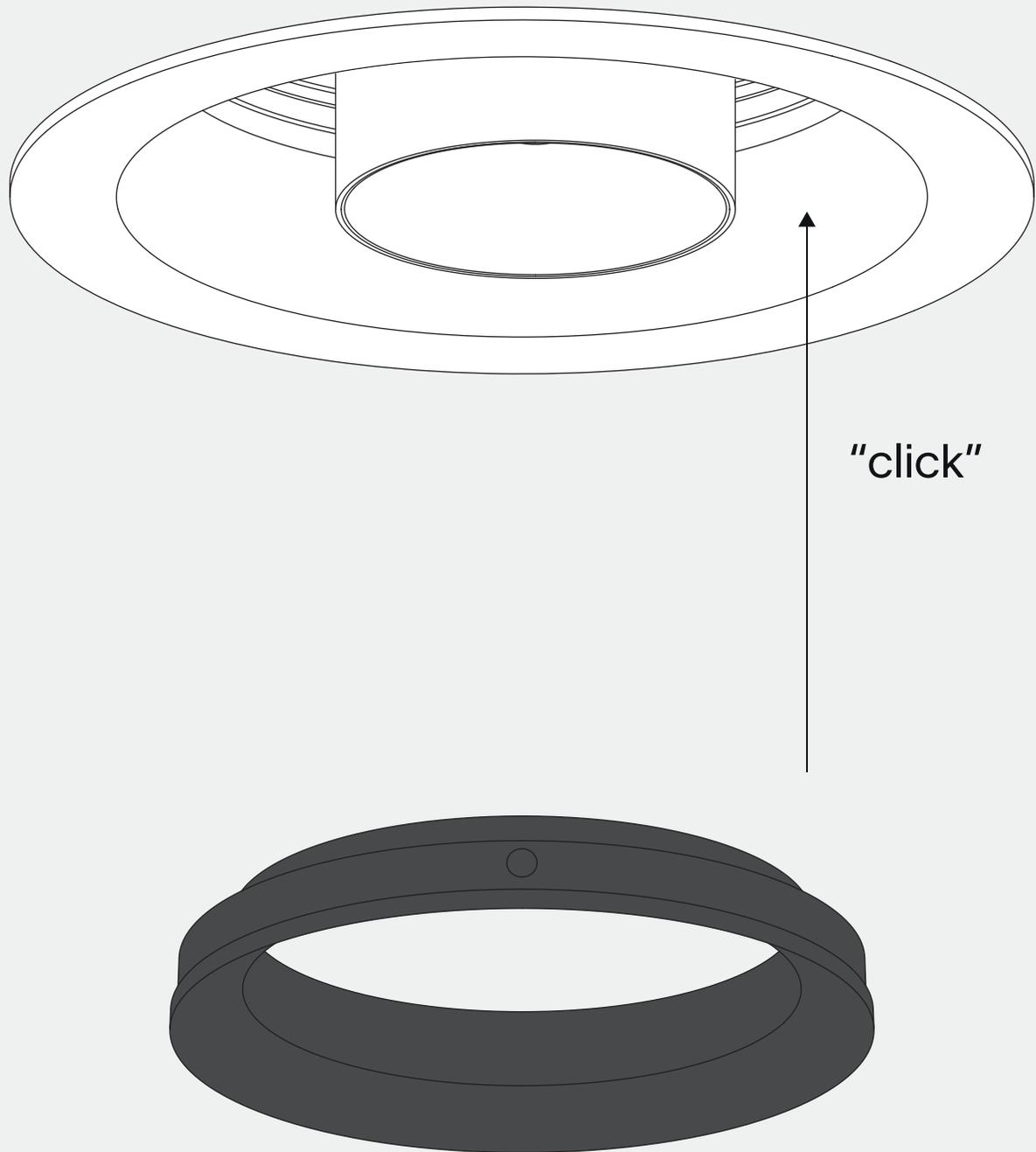
insert the design ring to lock the ventilation valve
