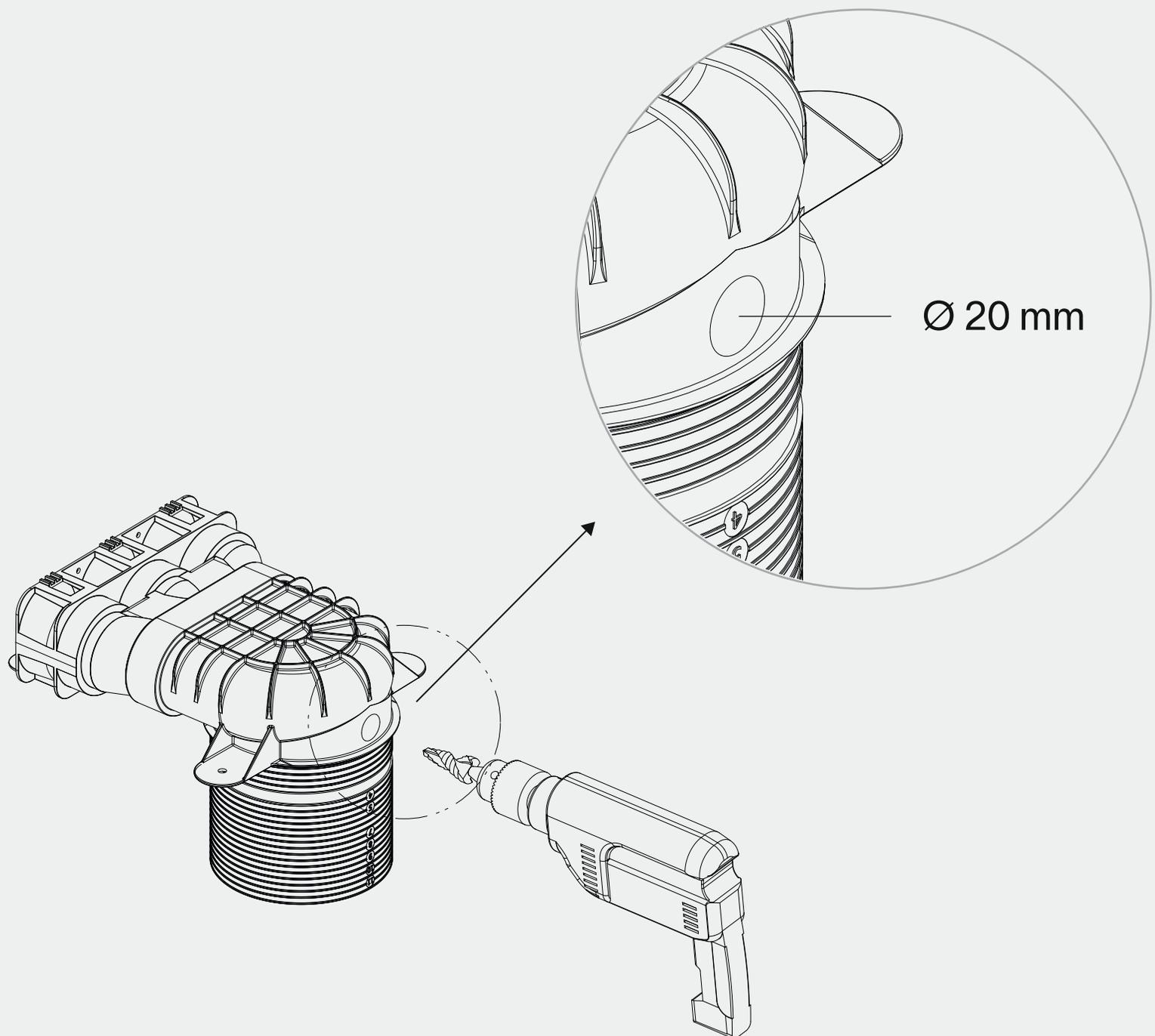
Use a step drill to cut a  $\text{Ø}20$  hole into the  $\text{Ø}125$  valve adapter of your choice. A hole can be drilled in any type or brand of  $\text{Ø}125$  valve adapter.
