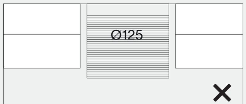
Cut off the excess length of the valve adapter.
