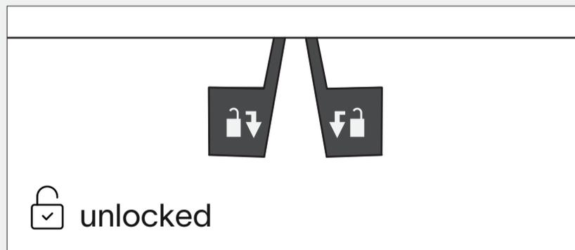
gently pull the lock out before adjusting the air flow
