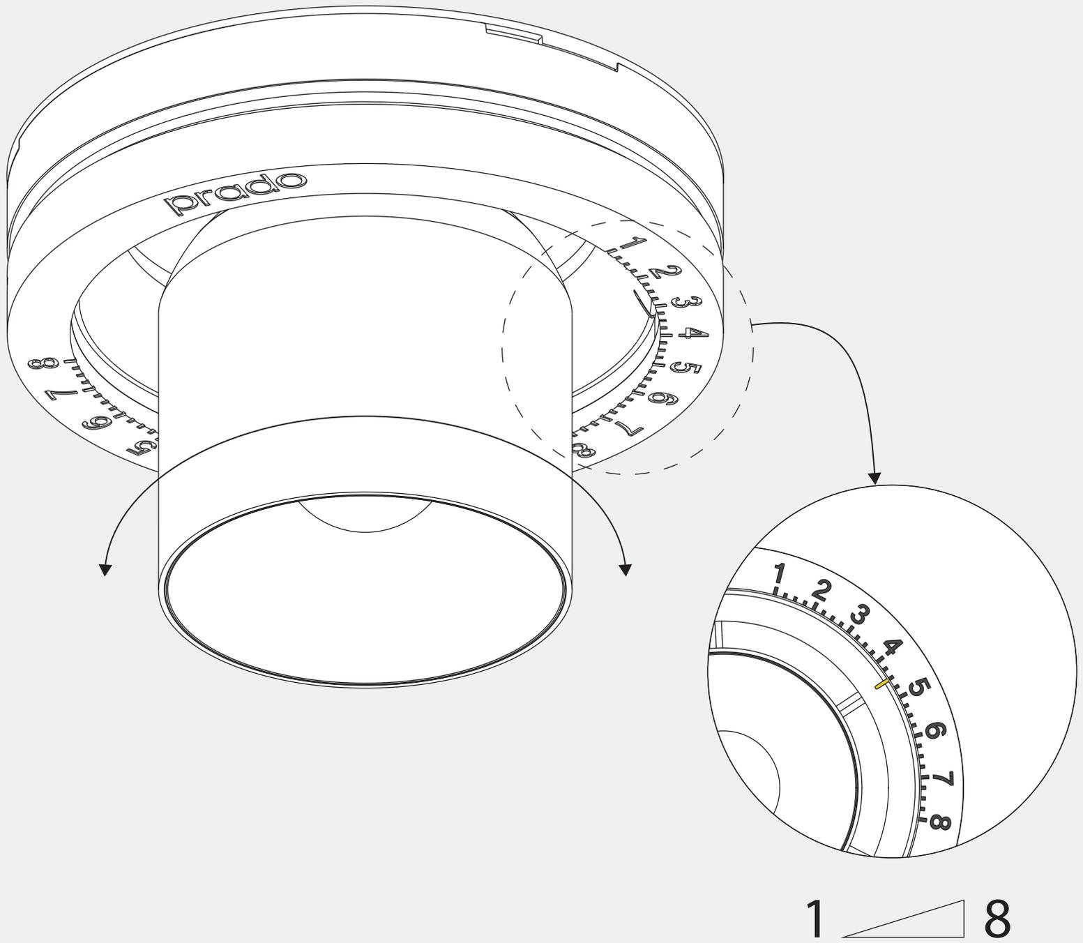
twist the luminaire to adjust the ventilation flow level
