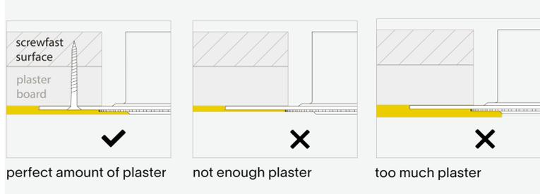
Excercise caution while plasing, do not damage the ring. Keep the plaster lid inside the plaster ring while plastering. Use a fiberglass mesh tape for optimal plaster adhesion. Make sure not to touch the edge of the ring when sanding.
