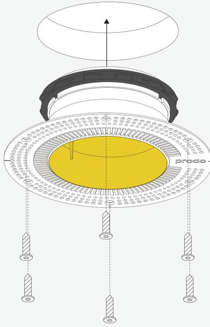
Insert the plaster ring and securely fasten it with glue or the appropriate screws on a screwfast surface. The attachment must be able to obtain a static load of 5 kg. It's the installers responsibility to ensure optimal attachment.
