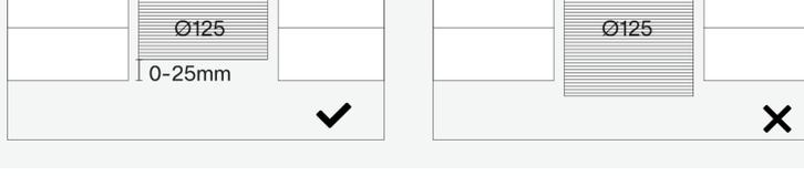
Cut off the excess length of the valve adapter. (between 0 and 25 mm above final ceiling level)
