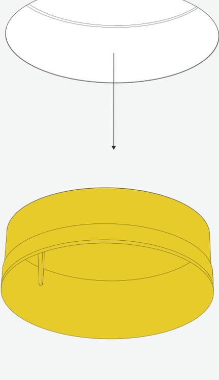
Remove the plaster lid just before installing the fixture. It helps to keep the inside of your plaster ring free of filler, paint and dust. Any residue needs to be removed without damaging the edges of the plaster ring.
