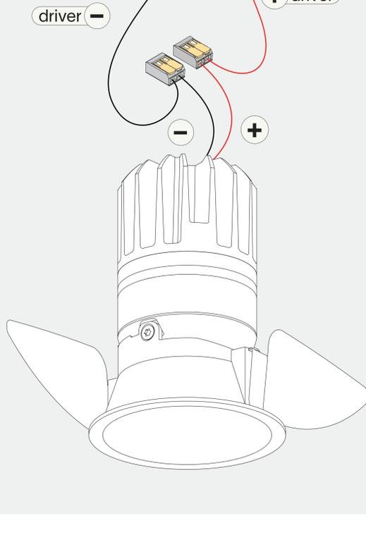
connect the wires with wago connectors for serial connection, respect polarity
