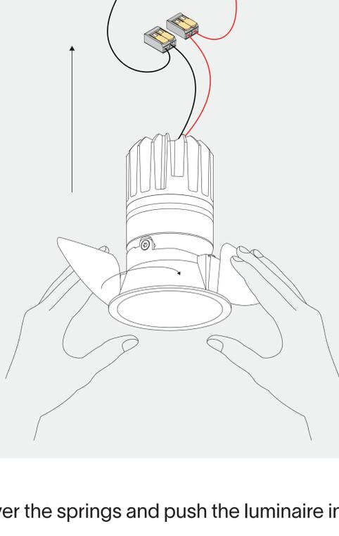
bend over the springs and push the luminaire into the ceiling
