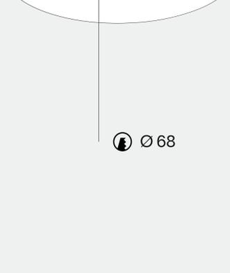
Cut a round hole (Ø 68). Consult the chosen luminaire tech specs for required height and free air dimensions.
