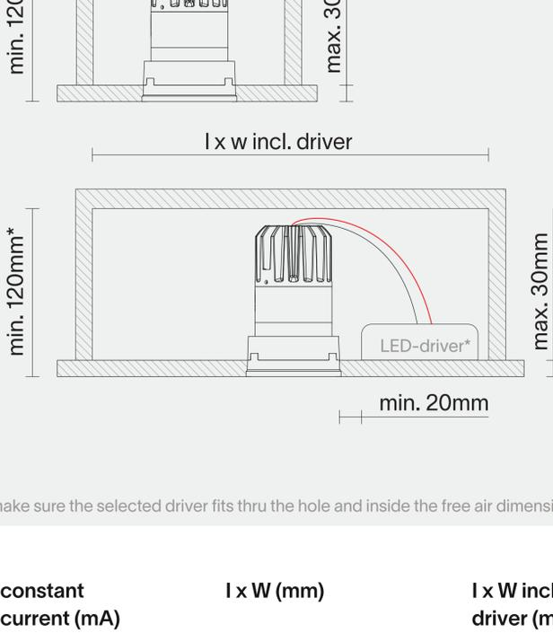
\*make sure the selected driver fits thru the hole and inside the free air dimensions
