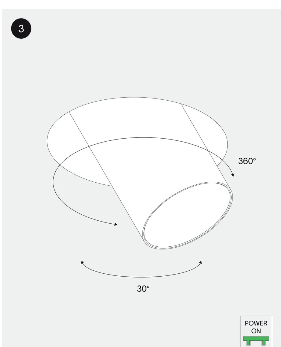
twist the luminaire as desired
