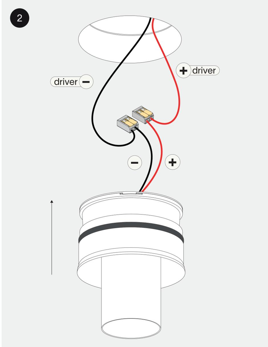
connect the wires with the connectors for serial connection, respect polarity combine with a prado LED-driver
