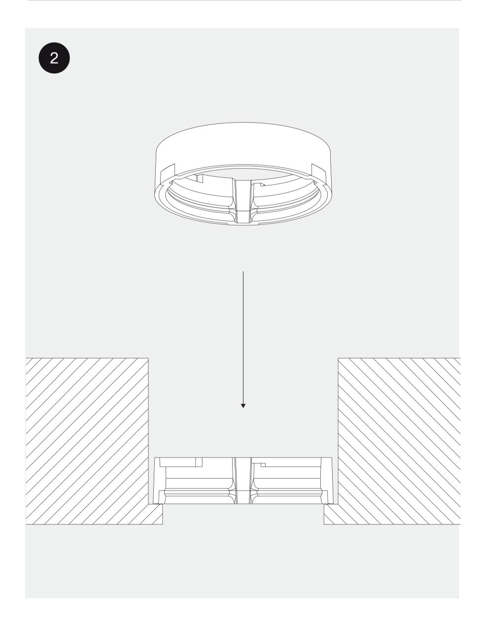
place the clt ring in the hole like shown above
