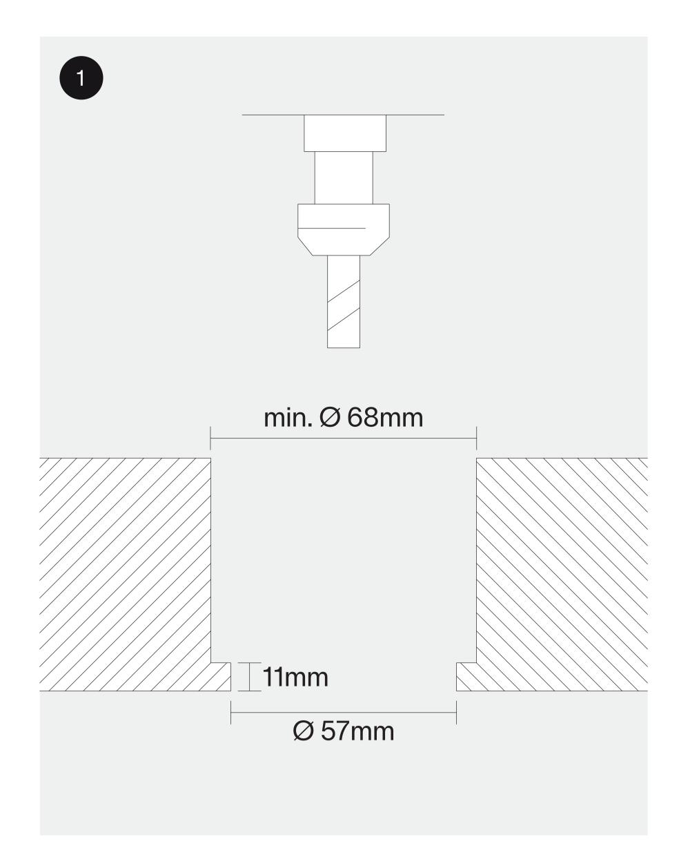
the chosen luminaire tech specs for required height and free air dimensions.
